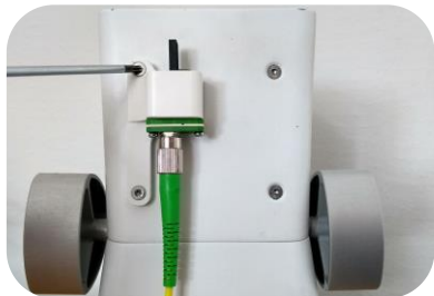
1. Mount the adapter with the two M3 screws on the back side of the Piuma head
