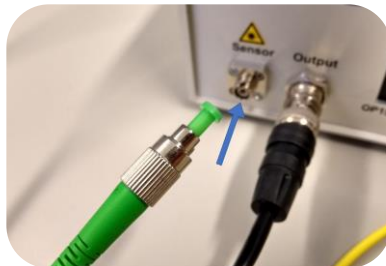
1. Connect one end of the patch-chord (old connector) to the OP1550
