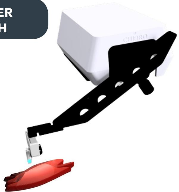
Figure 1. CHIARO Nanoindenter which can be mounted on an inverted microscope for single cell characterization. Not to scale.
