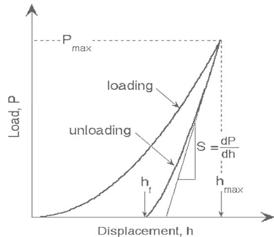
**Figure 2** – load-displacement curve
