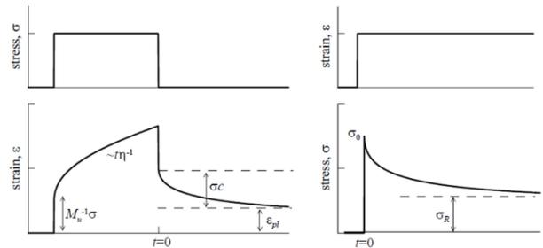
**Figure 3** – Schematic representation of creep (left) and stress relaxation (right) including important parameters.
