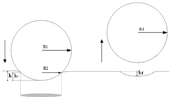
**Figure 1** – Schematic representation of sample indentation with a spherical indenter tip.
